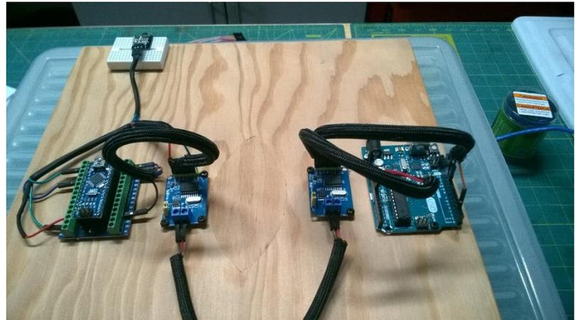
The typical circuit uses MCP2515\_CAN modules. The baud rate for the actual CAN bus is programmed into my transmitter sketch on the NANO. This demo is running at 500,000 bits per second.
