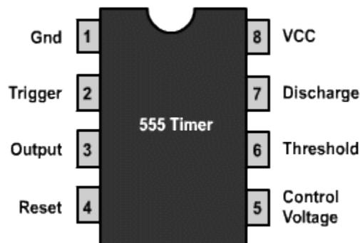
The chip can operate in one of two modes, depending on how the pins are connected.
