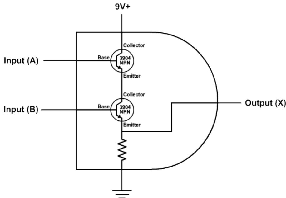
As the diagram indicates, the gate must receive electricity from a power source, and must also contain a ground, thus creating a complete circuit.
