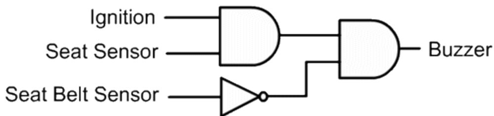
To see if this circuit achieves its desired output, a truth table can be used to trace the output for each possible input. In each row, a 0 represents “Off”, and a 1 represents “On”
