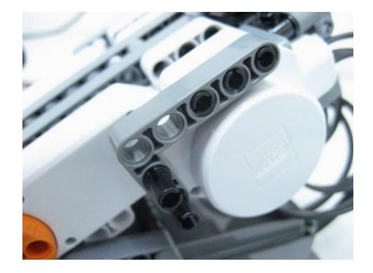
• Still on both sides, insert two black pegs in the two upper holes in the L-bracket.
