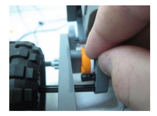
Once you've figured out where the wheel's axle should be, you can put this brace on so that the bottom hole holds the axle, and the black peg slides into the hole directly above the axle.
