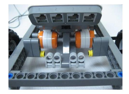
And here's what the frame looks like with two double-braces. With time and effort, you could use beams to connect the frame all the way across. If you did this, the frame would hardly bend at all.
