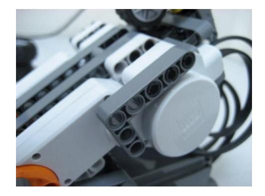
Next, on each side, attach the L-shaped bracket so that all three black pegs are covered. The upward leg of the bracket should face the front of the robot.
