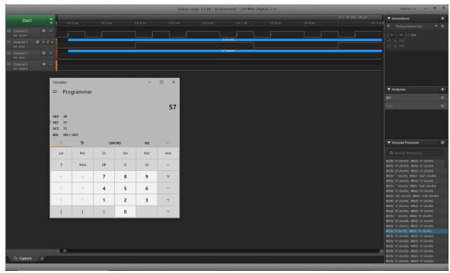
the LSB (0x39) packect. You can see the remaining data packets contain 0 because I did not transmit any more data. Although I could have made the remaining bits hold temperature or battery voltage if I needed to.
