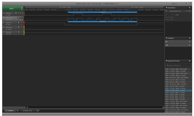
The most significant bit (MSB) is transmitted first (Big Endian).
