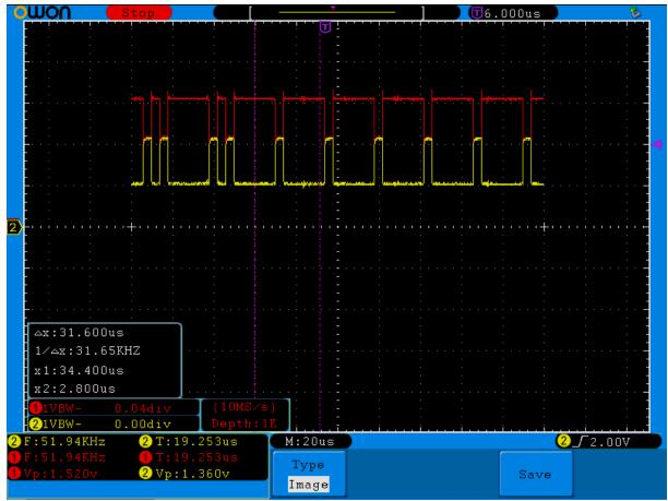
backwards doesn't it. These signals were collected with TWO terminating resistors on the Receiver & Transmitter nodes. The resistors are part of the CAN modules I am using. That measures 60 ohms across the H & L which is what you measure on an actual car.
