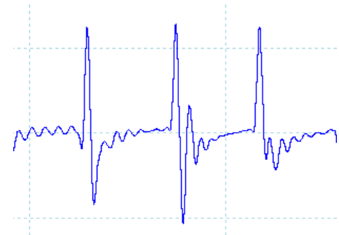
Figure 7: Knock Sensor Trace With 15Hz Low Pass Filter Installed
