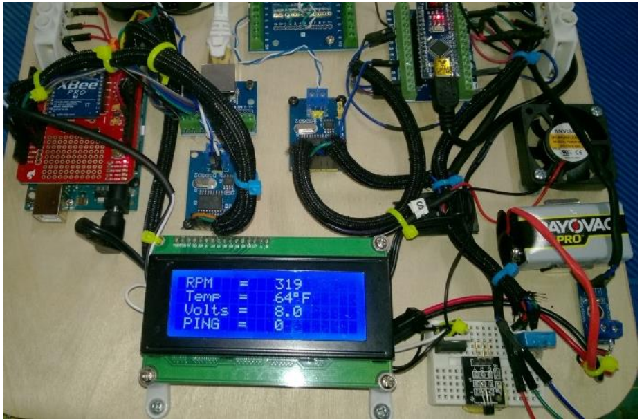
Figure 2: Canbus Setup Showing RPM
