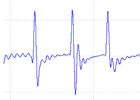
Figure 3-7: Knock Sensor Trace With 15Hz Low Pass Filter Installed
