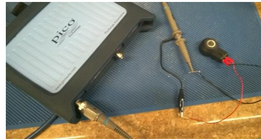
Figure 3-3: Bench Testing the Knock Sensor
