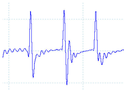
Figure 3-7: Knock Sensor Trace With 15Hz Low Pass Filter Installed
