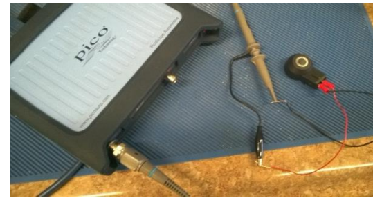
Figure 22-3: Bench Testing the Knock Sensor
