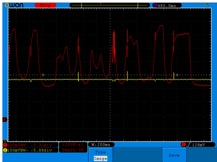
Figure 7 Excessive noise from LDR when signal is near reference voltage
