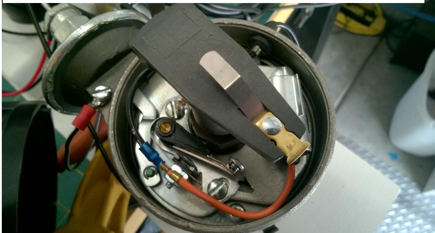
Figure 3: This shows the rotor. It takes the high voltage from the coil (center of distributor cap) and distributes it to each plug.
