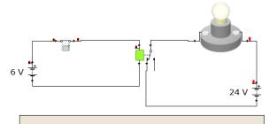
When the switch is closed, the rely is energized. Notice the contact points are closed open and the lamp receives power.
